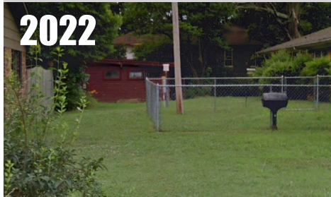
Updated to MMTS and moved to a new location, now closer to buildings and more wind sheltered than before. RATING = CRN4
