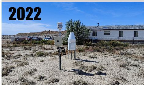
Site moved, new wireless MMTS provided. Better location. NWS reports: "SITE MOVED 1.99 MILES EAST SOUTHEAST" RATING = CRN2
