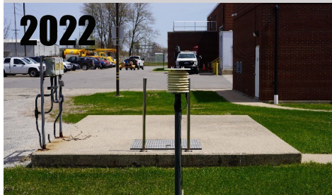
Same location at WWTP, but moved and converted to MMTS. Slightly better siting compared to original location. RATING = CRN4
