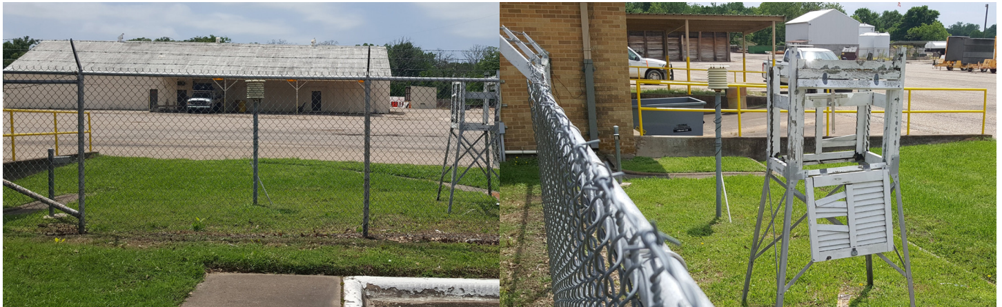
MMTS and CRS, at a GHCN station in the Paris, TX, city maintenance yard. Heat sinks surround this station. Source: H. Sterling Burnett.
