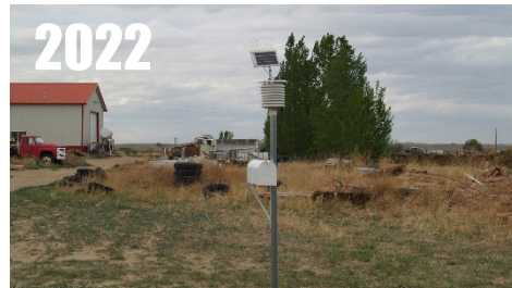
Moved, but new station is compromised by addition of mailbox and solar panel. RATING = indeterminate, there is no formula for mailboxes.
