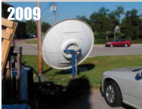
Troy, AL , nearby parking lot, MMTS at rear of satellite dish. RATING = CRN4
