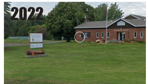
Same location, but CRS upgraded to MMTS and moved to front lawn. Better siting, but still only 25' from brick building. RATING = CRN4
