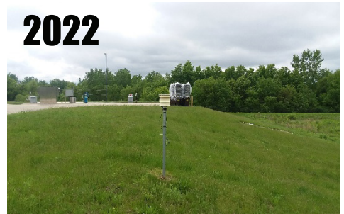
Same location at city WWTP, but moved away from tanks when converted to MMTS. RATING = CRN3
