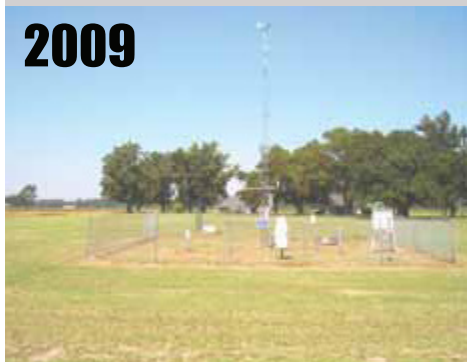
St. Joseph, LA , well-sited station. RATING = CRN1
