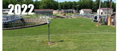
MMTS was moved to a somewhat better location at city WWTP. NWS reports: "RELOCATED STATION 2 MILES SOUTHEAST OF PREVIOUS SITE, TO THE PARIS SEWAGE TREATMENT PLANT." RATING = CRN3
