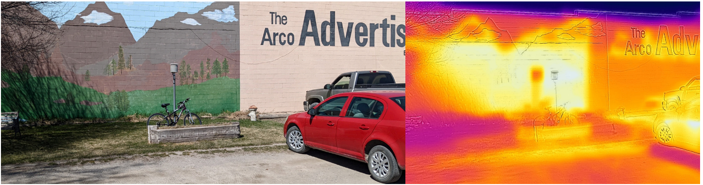
Visible and infrared photos of MMTS placement near sunlit wall and large parking lot at Arco, ID, GHCN Station. Source: Anthony Watts.
