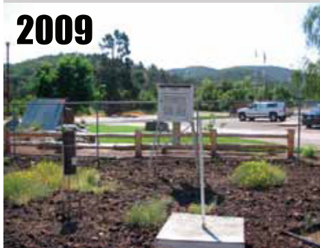
Yreka, CA , CRS sited on cinder rock, nearby concrete driveway, parking lot, road. RATING = CRN5
