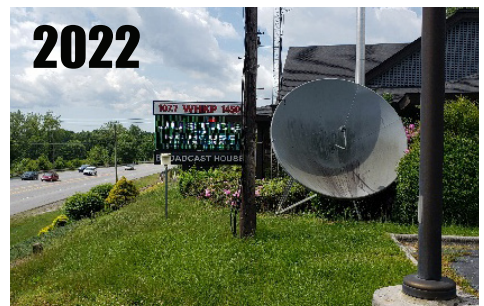
Location unchanged, but MMTS moved about 15 feet away from parking lot. Improved siting. RATING = CRN4
