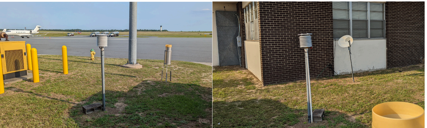
MMTC placement at the airport fire station in Tallahassee, FL, a GHCN station. Note the proximity of multiple heat sources and sinks. Source: Anthony Watts.
