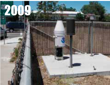
Paso Robles, CA , sited on concrete slab next to sidewalk, nearby road, interstate. RATING = CRN5
