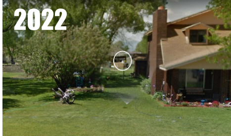
Station closed, moved to private residence. Siting is better than a parking lot, but has issues with shading and irrigation. RATING = CRN4
